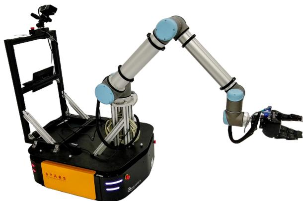
Figure 2.6: The mobile manipulator used to perform the experiments in this thesis. It consists of a Clearpath Ridgeback mobile base, UR10 arm, Robotiq FT-300 wrist-mounted force-torque sensor, and Robotiq 3-finger gripper. The planar pose of the base is tracked with a Vicon motion capture system.
